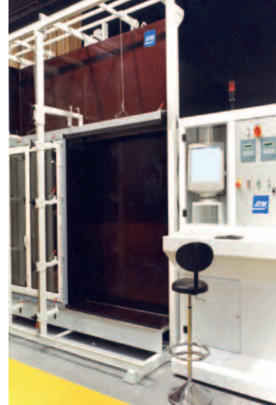
Banc Essais Air-Eau-Vent (AEV)
